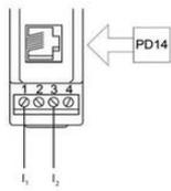
d) indirect measurement of current by means of current transformer
