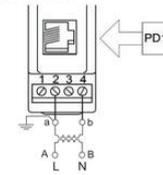
c) direct measurement of current
