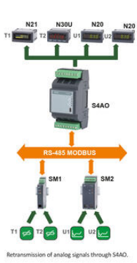
Increasing number of analog outputs in power network meters by adding S4AO module.
