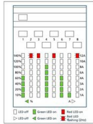
Fig. 7-2: LED Light pattern in measurement mode
