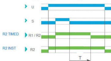
Function C - Off-Delay (Delay on break)
