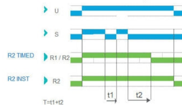
Function Ht - Interval summation time relay
