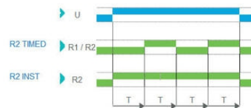
Function D - Symmetrical flashing (OFF Start)
