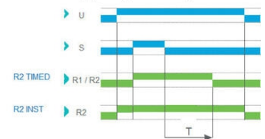
Function C - Off-Delay (Delay on break)
